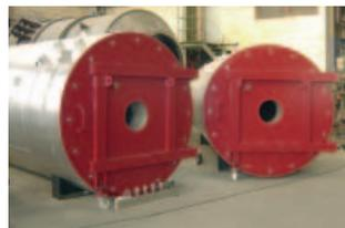
Thermal oil heater fired with natural gas and/or heavy oil, used for a polyester production plant in Thailand, with a capacity of 3 MW
