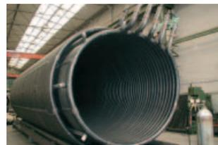
Waste heat boiler in three-pass design with a net capacity of 8 MW, for heating of a production line for rubber products
