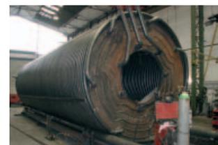
Radiation boiler with built-in opening for dust burner, with oil-cooled combustion chamber cover
